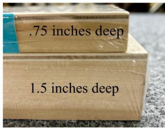
Top example requires framing Bottom example requires solid edge as specified above.
